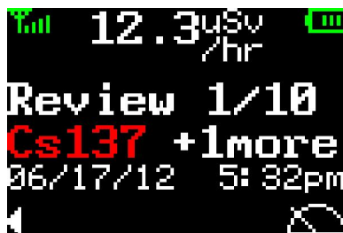
Figure 18 - Review screen showing the first of ten sets of measurements. In addition to CS137, one more radioactive substance has also been identified.
