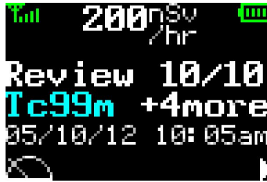
Figure 19 - Review screen showing the tenth of ten sets of measurements. In addition Tc99m, four more radioactive substances have also been identified.
